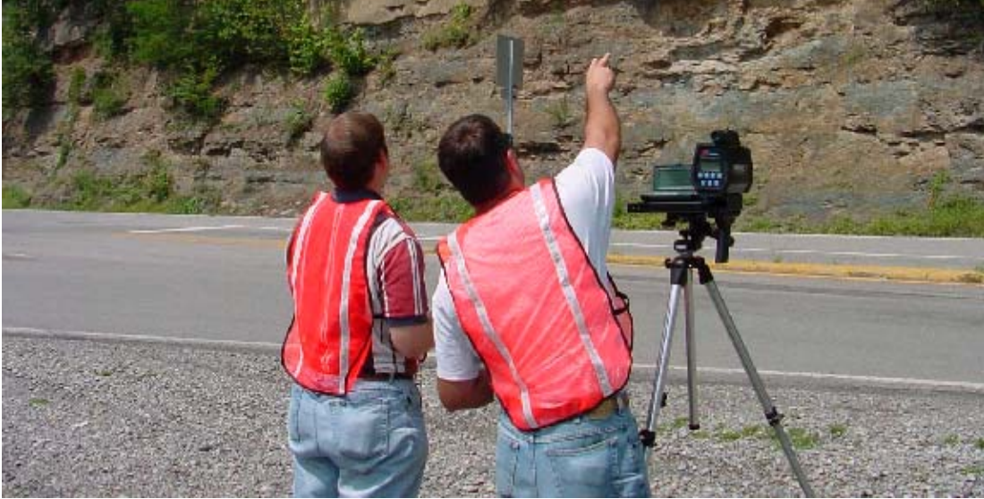
Figure 2: Using the laser gun and slope profiling instrument.
