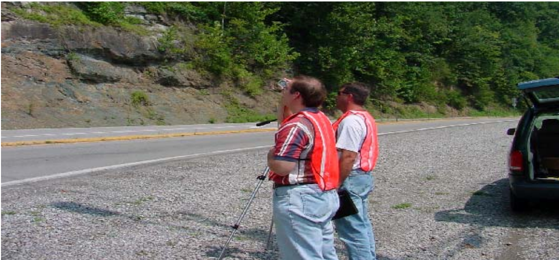
Figure 1: Determining the rock slope height using an inclinometer.
