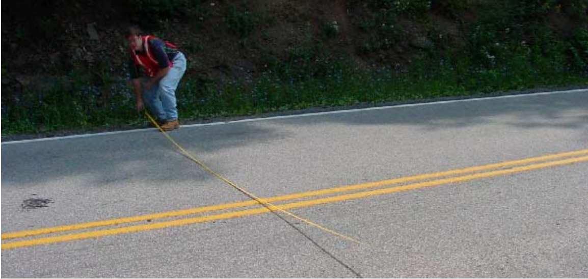
Figure 5: Measuring the width of road.
