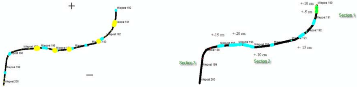
Figure 4 Illustration of track displacement between two GNSS surveys across a ten-mile segment. Horizontal displacement greater than 0.5 feet – left, vertical displacement over 0.5 feet – right.
